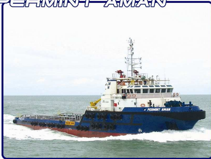
STRAIGHT SUPPLY VESSEL FIFI 1 BHP 4600
