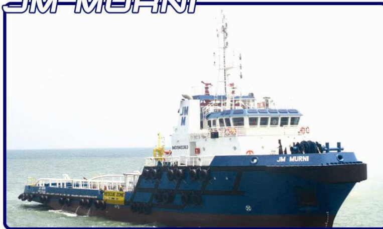
STRAIGHT SUPPLY VESSEL, 4640 BHP x FIFI 1
