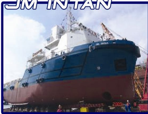
60 M ANCHOR HANDLING TUG - SUPPLY VESSEL FIFI BHP 5220 BHP 65 T BOLLARD PULL
